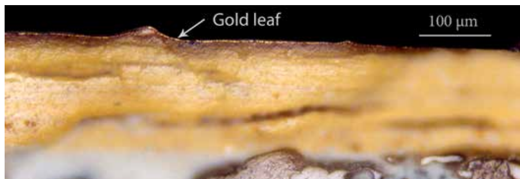
Fig. 5. Aigai, Museum of the Royal Tombs. Chryselephantine couch from the burial chamber of the tomb of Philip II. Photomicrograph of paint cross section in reflected light. In the sample are visible four distinct layer: a white layer of kaolinite/calcite; a layer of yellow ochre; a thin semi-transparent layer of an organic binder and a gold leaf. © H. Brecoulaki.
